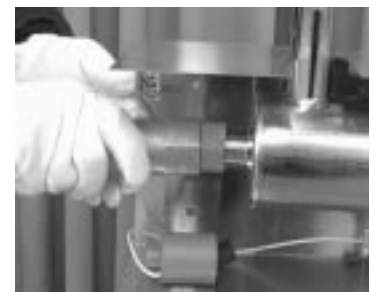
Rotate compression nut clockwise
