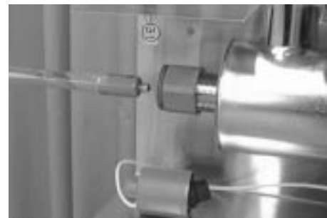
Step 5: Insert lamp into quartz sleeve.
