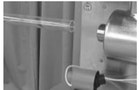
Insert quartz sleeve into threaded nipple.
