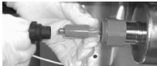
Step 8: Slide boot onto lamp socket assembly.
