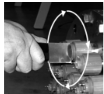
Rotate compression nut clockwise onto the threaded stainless nipped end plate with compression nut tool
