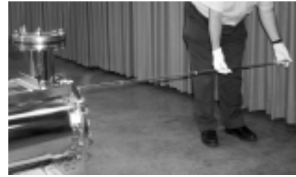
Insert the lamp in a level, horizontal position.
