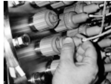
Secure lamp socket connector to lamp
